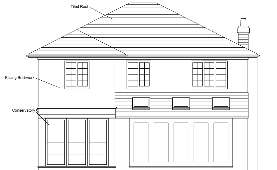
Existing Rear Elevation
