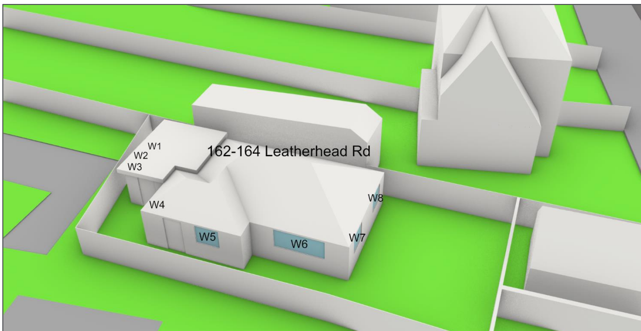
Figure 12 - Illustration of window openings at 162-164 Leatherhead Road (view from south), without overhangs
