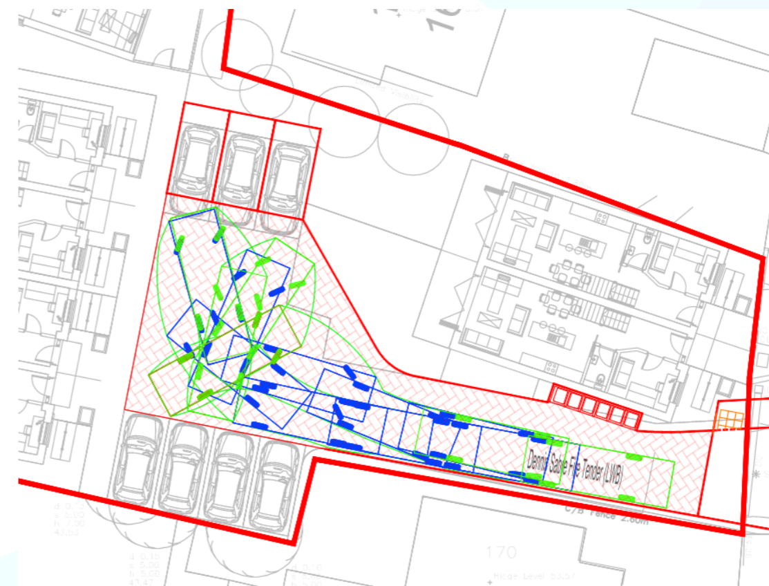
Figure 10 – Fire tender turning within the car park
