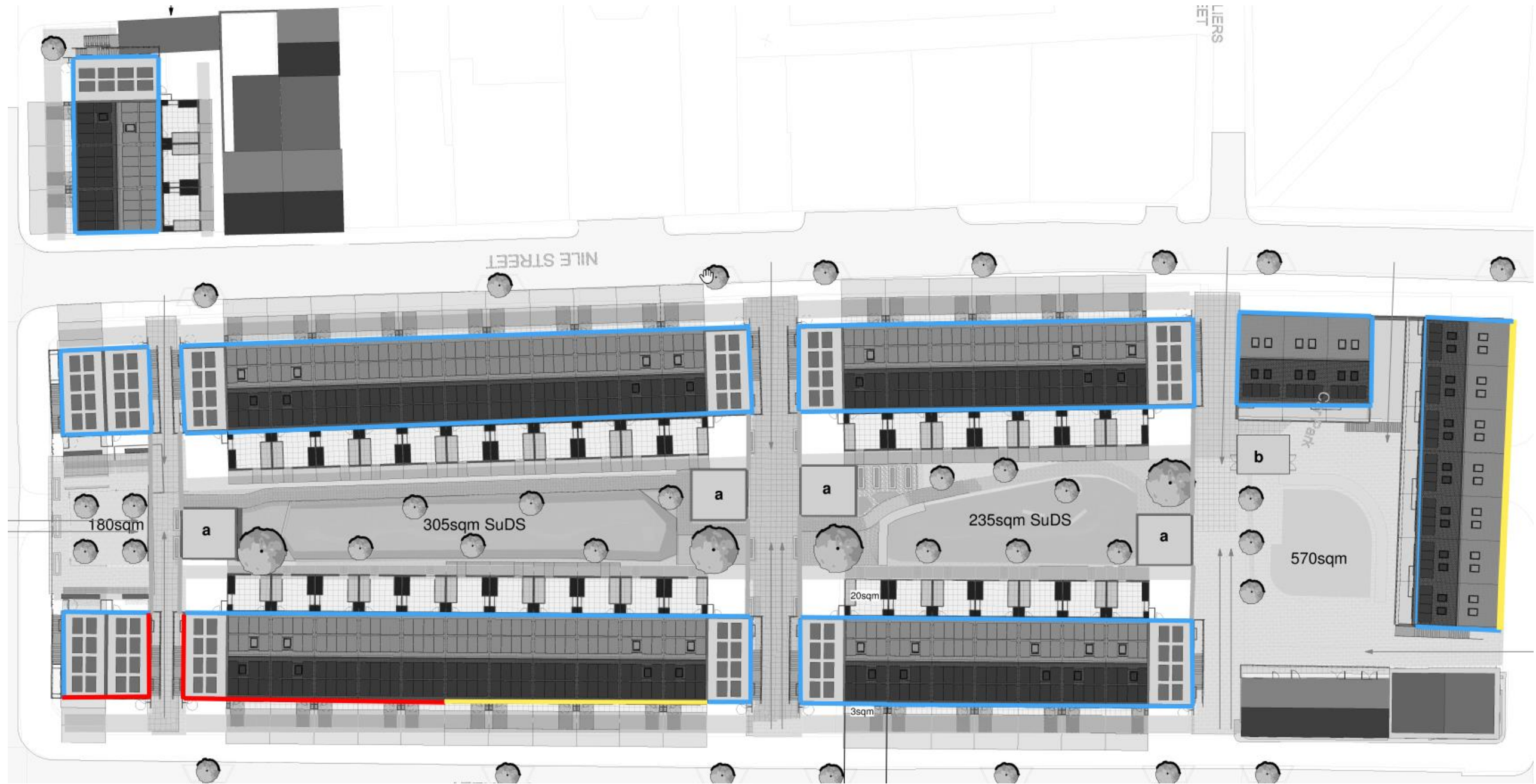
Figure 1: Façade sound insulation mark-up
