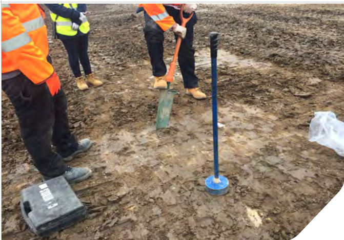
Photo 05: Core cutter test, zone 7 layer 1.
