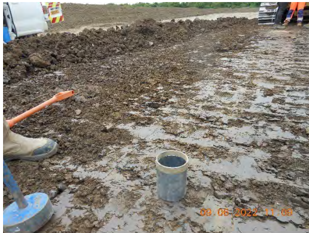
Figure 7. Core cylinder and dolly prior to embedment with ram.
