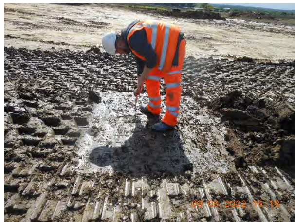
Figure 31. Shear vane testing on completion of passes five and six of layer two.
