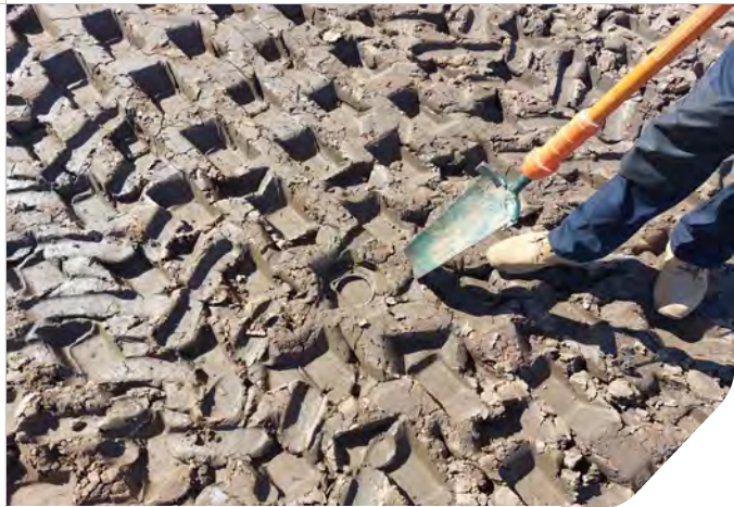
Photo 03: Exploration testing engineer undertaking core cutter tests in Zone 8
