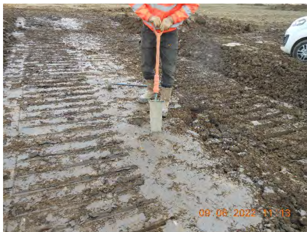
Figure 8. Digging out core sample cylinder.
