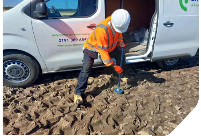
Photo 02: Exploration testing engineer undertaking core cutter tests in Zone 8
