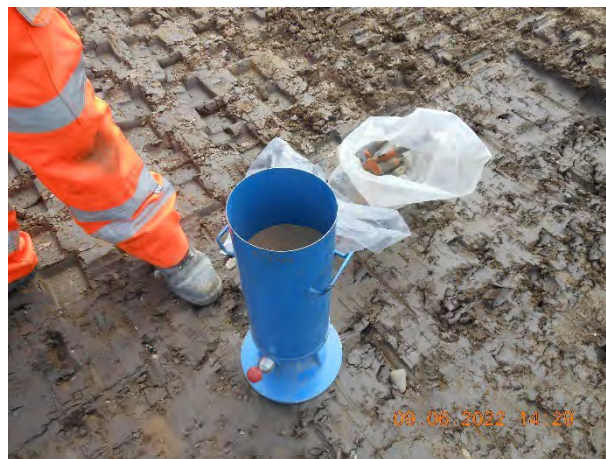
Figure 22. Sand in cylinder prior to sand replacement test.
