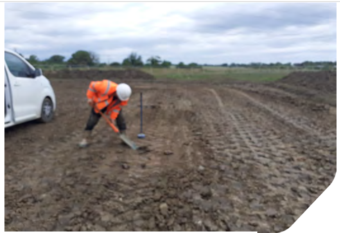
Photo 08: Removing Core Cutter
