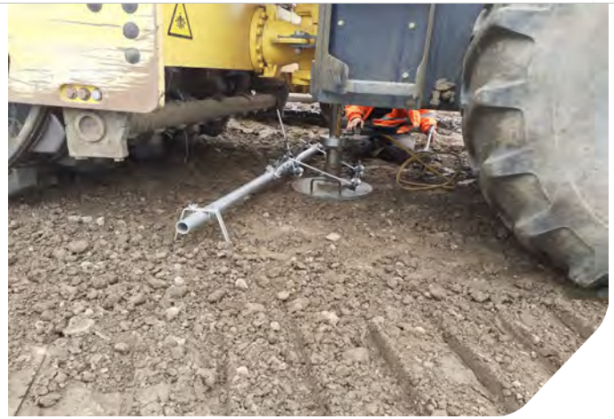
Photo 04: Plate Load Testing
