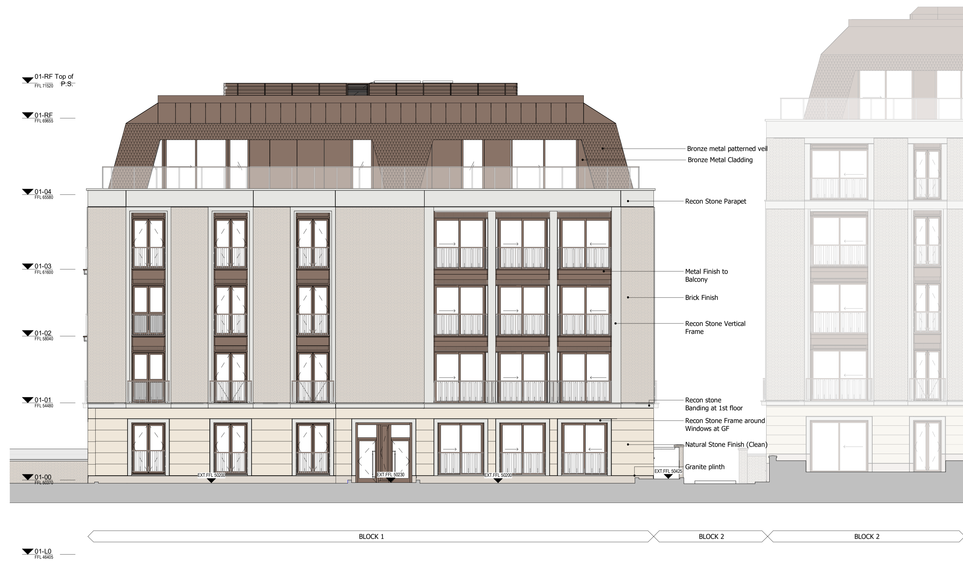
1 Block 1 - North East Elevation 1:100
