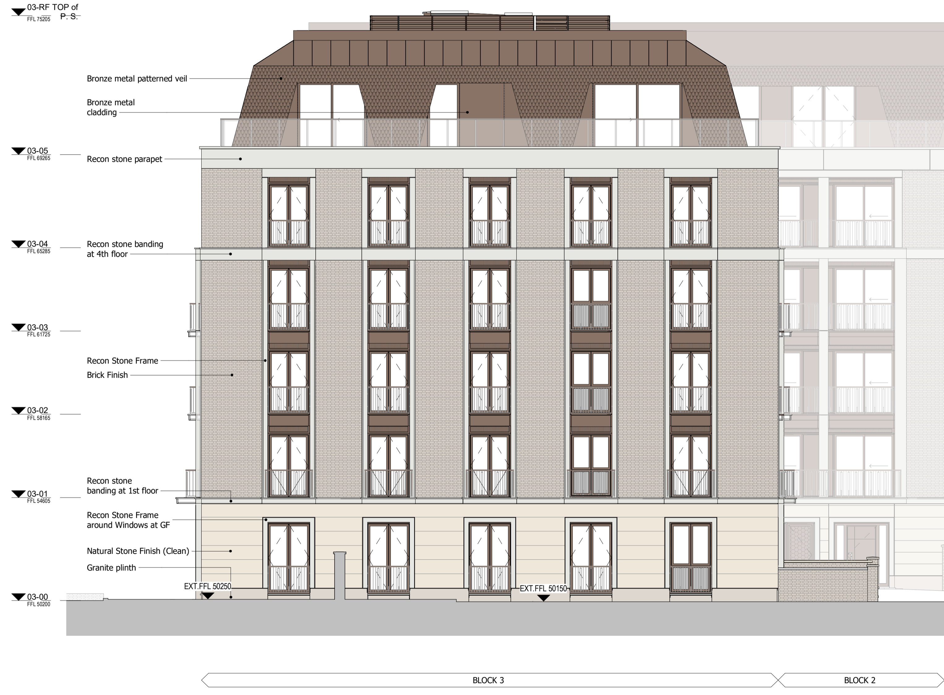
1 Block 3 - North East Elevation 1:100
