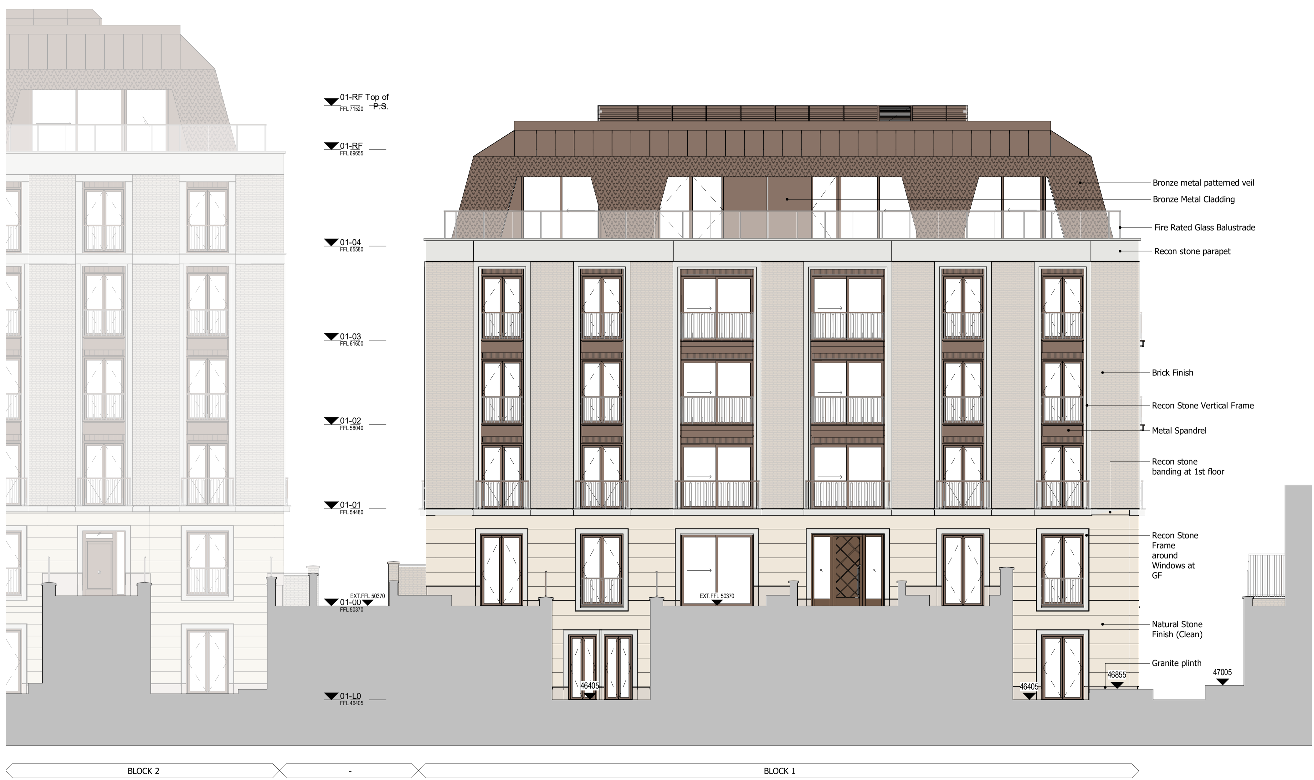
1 Block 1 - South West Elevation 1:100
