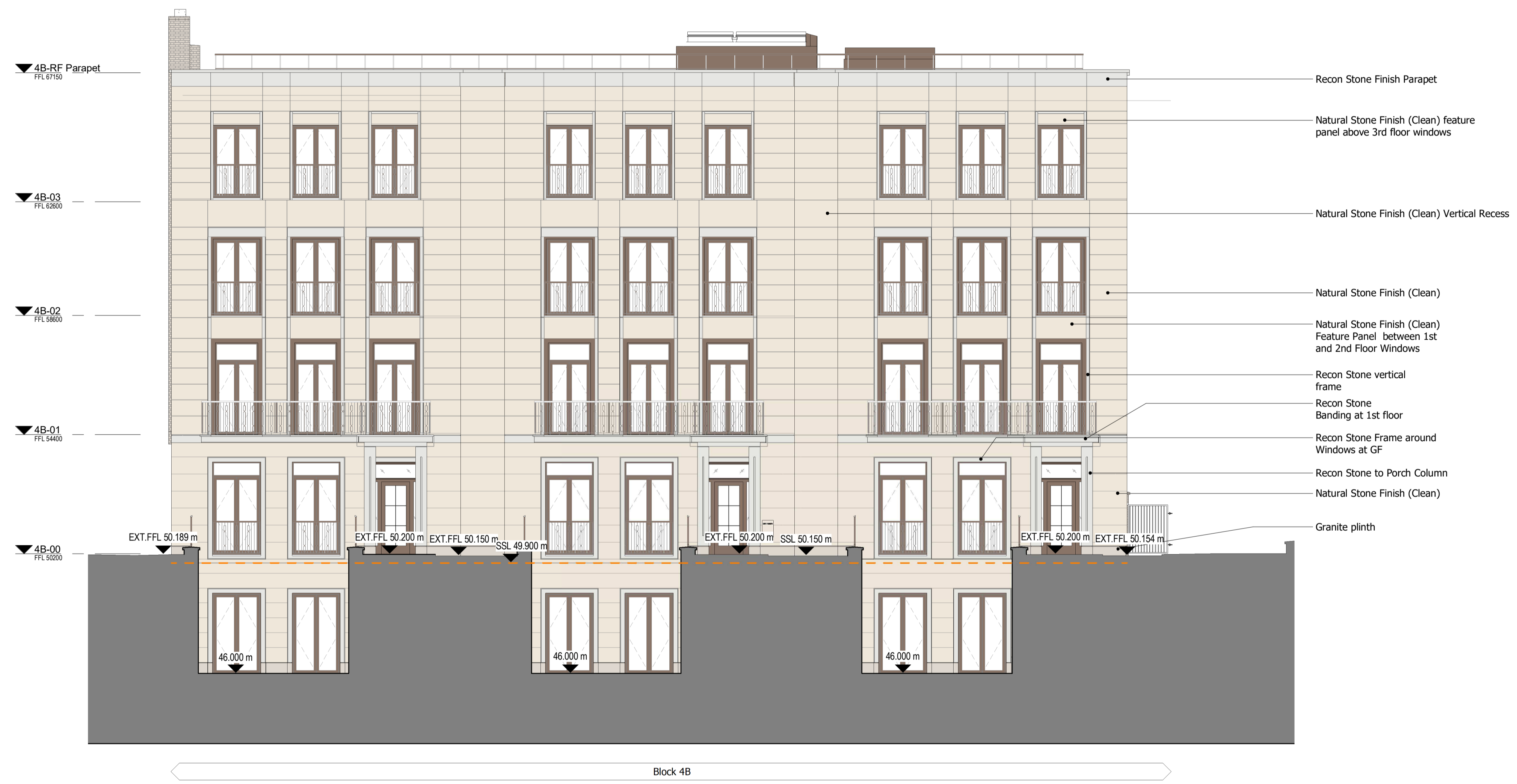
1 North West Elevation Finishes 1: 100
