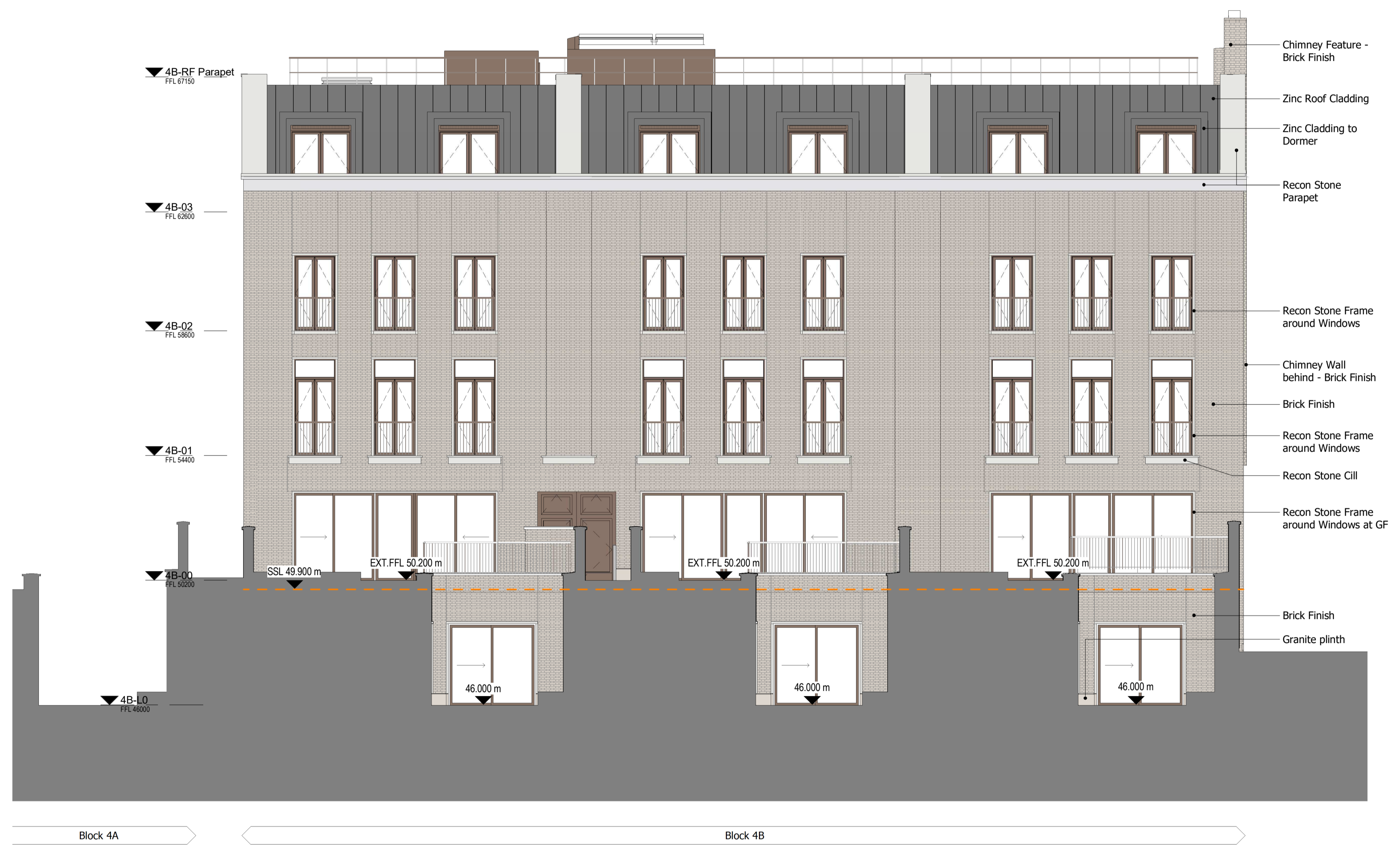
1 South East Elevation Finishes 1:100
