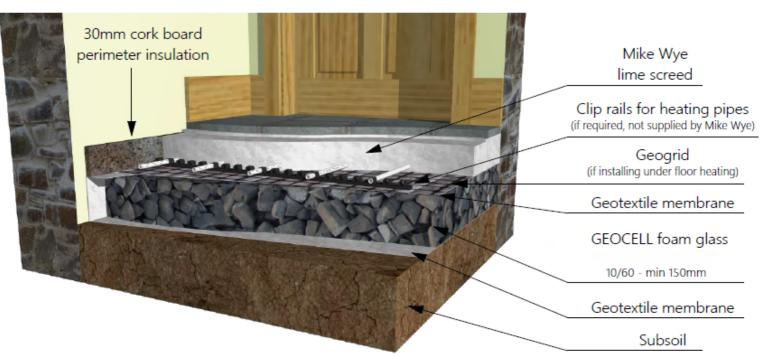
When the existing floor has been removed, excavate (if required) to the depth as calculated by Mike Wye Ltd, taking care not to undermine foundations. Accurately level and compact the surface, variations in levels can significantly increase material consumption.
