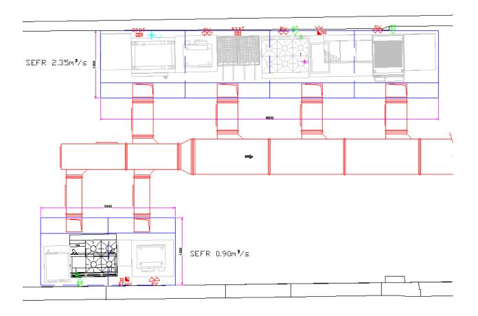
For the main canopy, the Specific Extract Flow Rate (SEFR) was calculated at 2.35m<sup>3</sup>/sec using the Thermal Co-efficient Method as advised by DW/172:2018. See accompanying SEFR calculation sheet.
