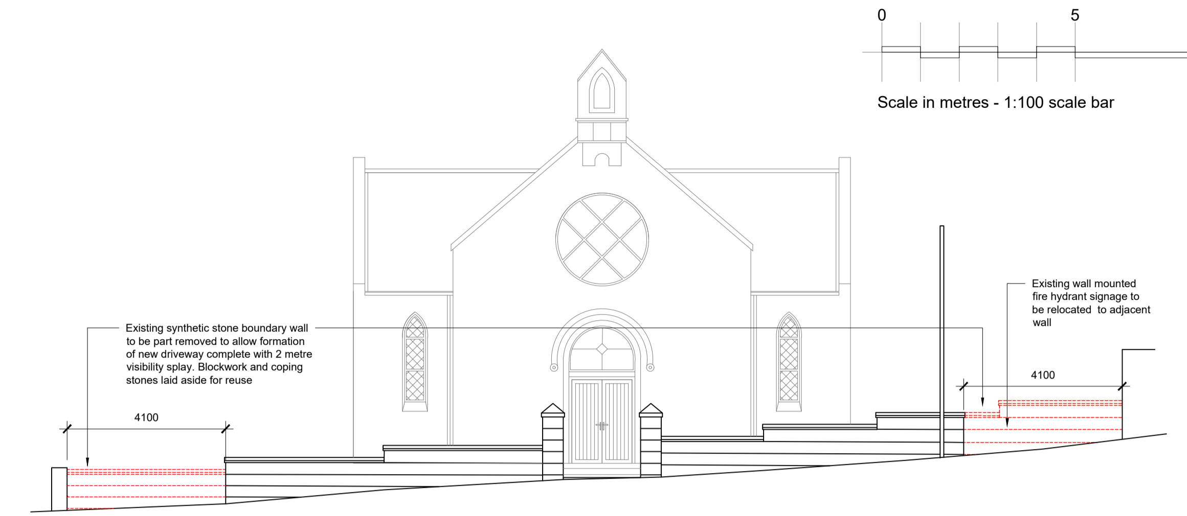
PROPOSED NORTH FACING BOUNDARY WALL Scale 1:100
