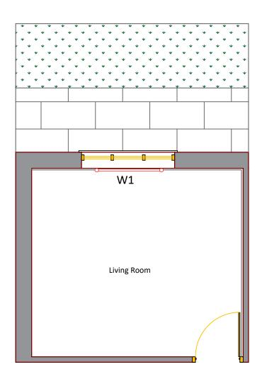
**NEW FRENCH DOOR**: Supply and install a 1 x new PVCu french doors New D1 as indicated on drawing with level access cills at base (Storm guard or similar type style level access cill) Externally the cill shall be installed to make the doorway as accessible as possible for a disabled user. Supply and fit suitable lintel for nature of work.
