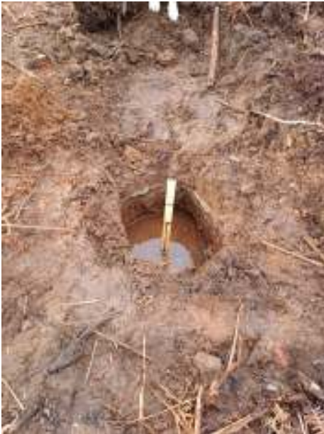
Photo 3 Showing Percolation Testing
