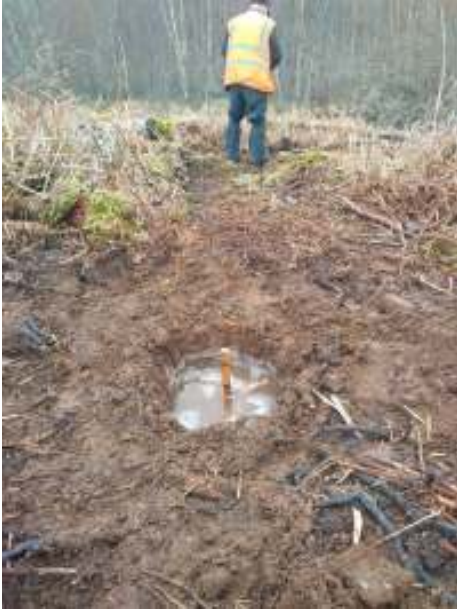
Photo 2 Showing Percolation Testing
