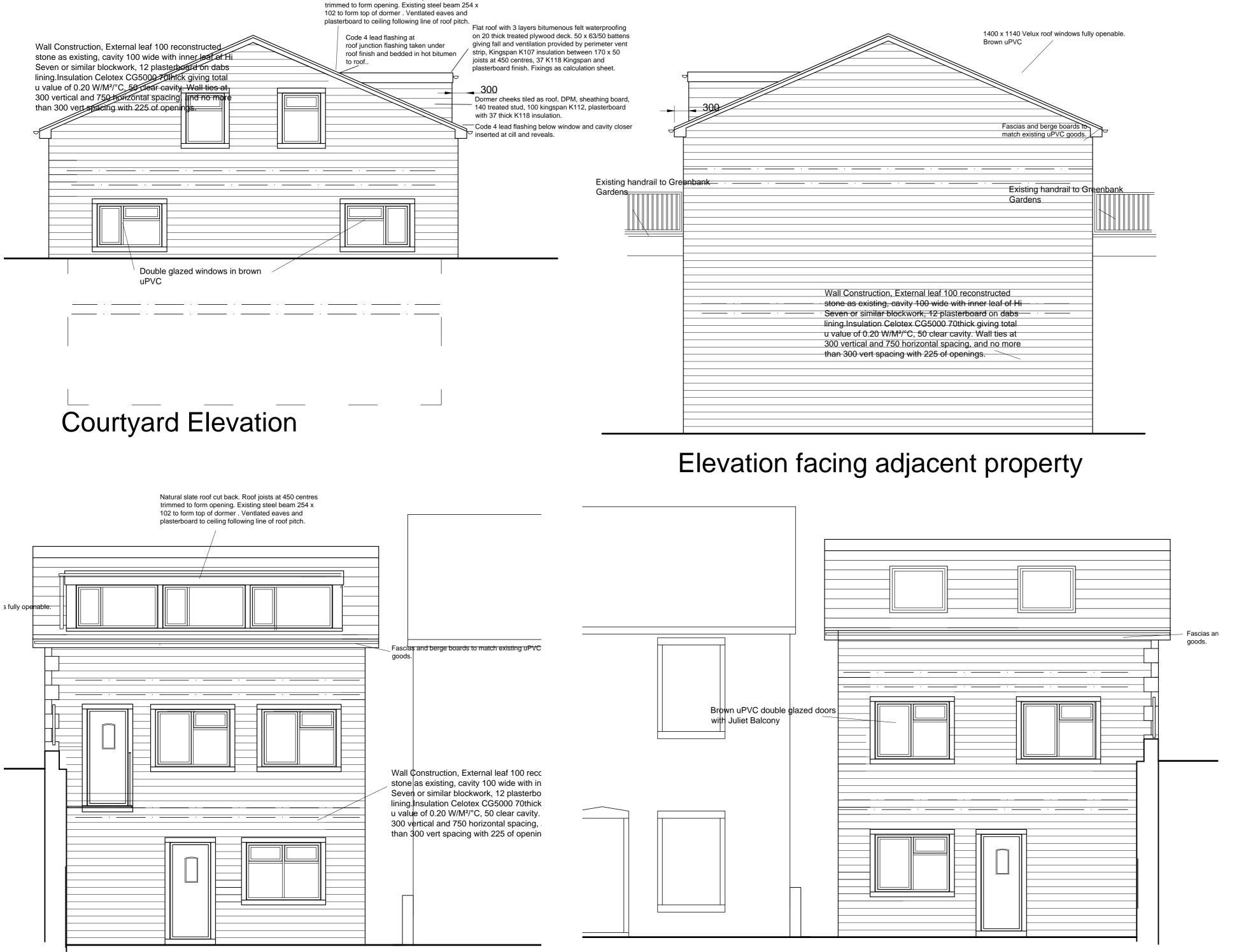
Natural slate roof cut back. Roof joists at 450 centres
