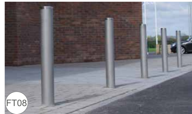
Manufacturer: Hartecast Ltd Product reference: HC2065P removable bollard Material: 316 grade Stainless steel Finish as delivered: Polyester powder coated with polished cap Colour: TBC Height above ground: 900mm Overall height (above and below ground): 1200mm as per manufacturer's standard design. Sectional size: 114mm diameter
