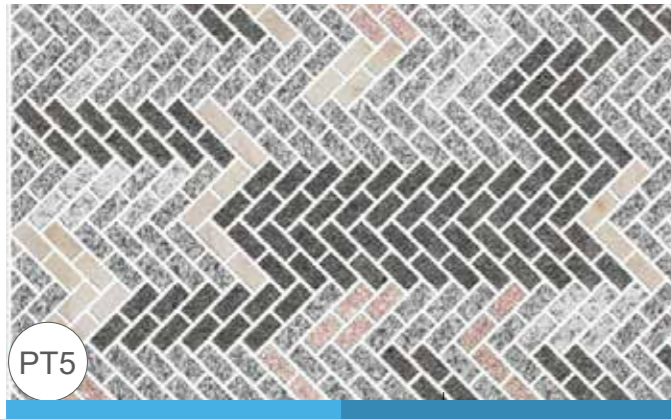
PT5 Supplier: Marshalls Product: Granite Sett Paving Size: PT5a 300x 150mm (Depth: 80mm) PT5b 200 x 100mm (Depth 60mm) Colours: mix Finish: Fine Picked Bond: Herringbone
