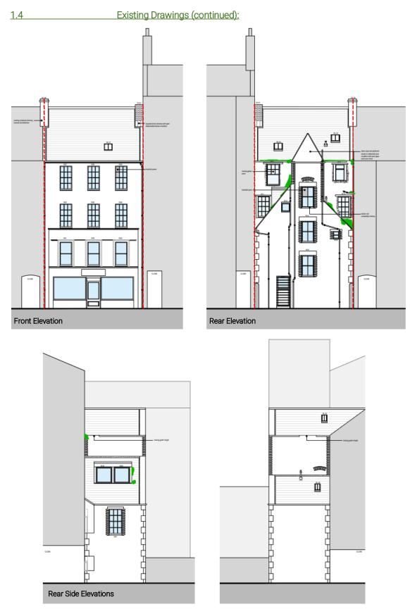
The elevations, shown above, shows the pediment to the rear elevation with two lower roofs to either side as well as a dormer to one side. The green areas on the drawings highlight the significant vegetation growing on the stone.
