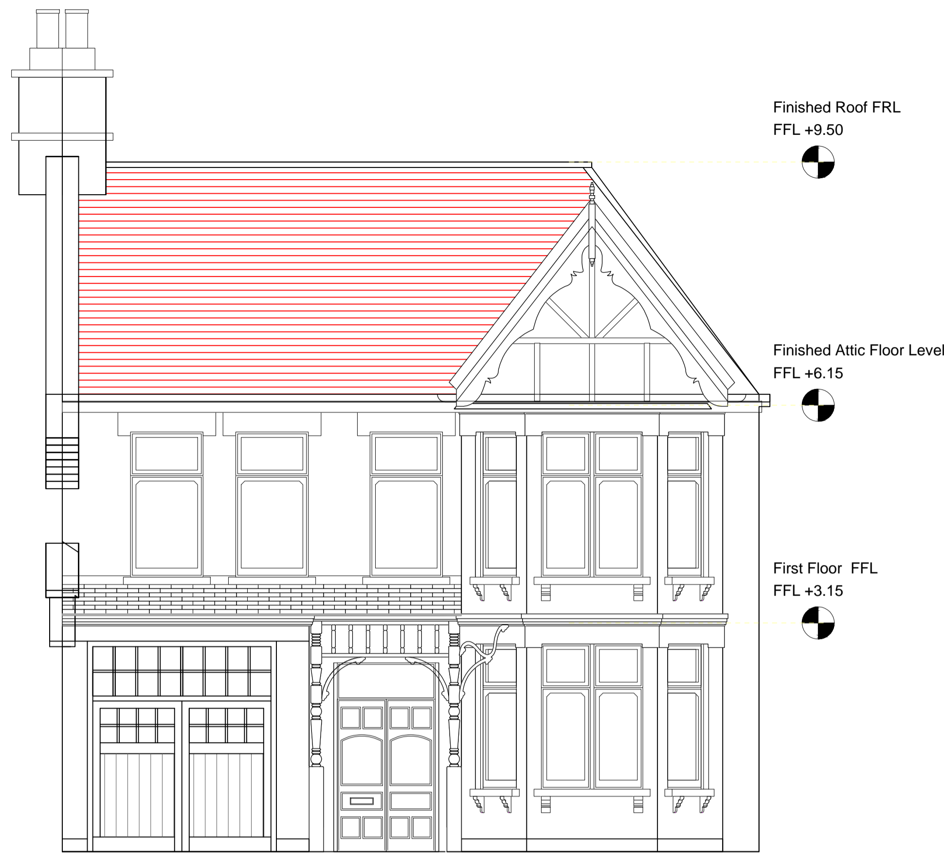
EXISTING FRONT ELEVATION
