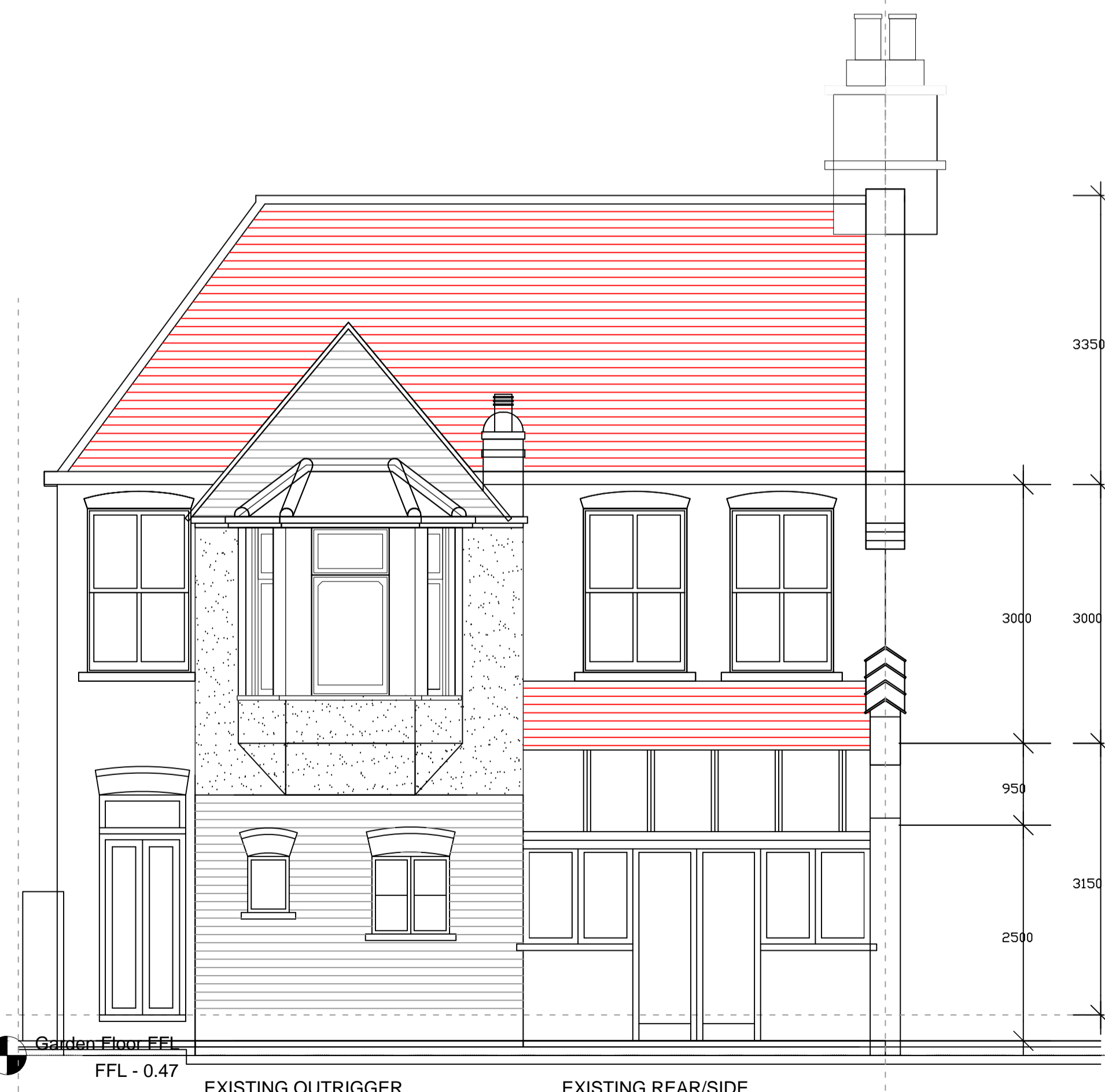
EXISTING REAR ELEVATION
