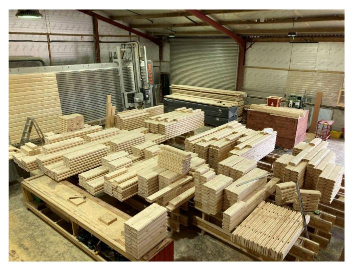
All components have identity markings corresponding to the installation plans, providing the manufacturing operatives the information required to assemble the mobile home or twin unit caravan.
