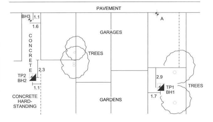
Note: Fourth borehole at position 'A' could not be commenced due to encountering buried old wall footing or similar.
