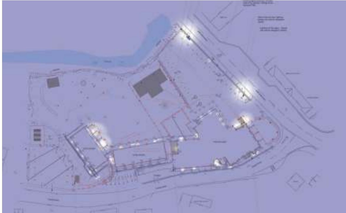
Illustration of current lighting scheme - provided by a range of light fittings and two street lamps on A466. (For comparison purposes this illustration uses the exterior services plan and shows lighting that is mounted under first storey building canopies).
