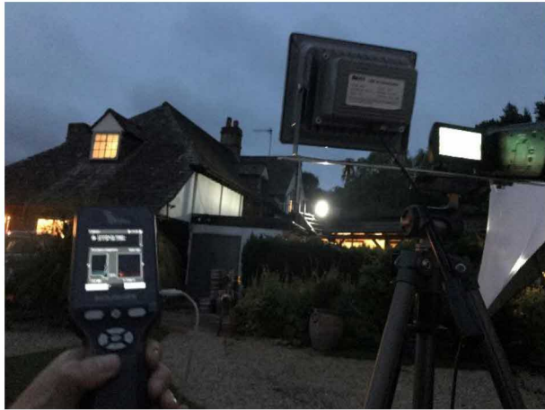
Photograph A2.1: Infrared camera set up outside building B1 during emergence survey
