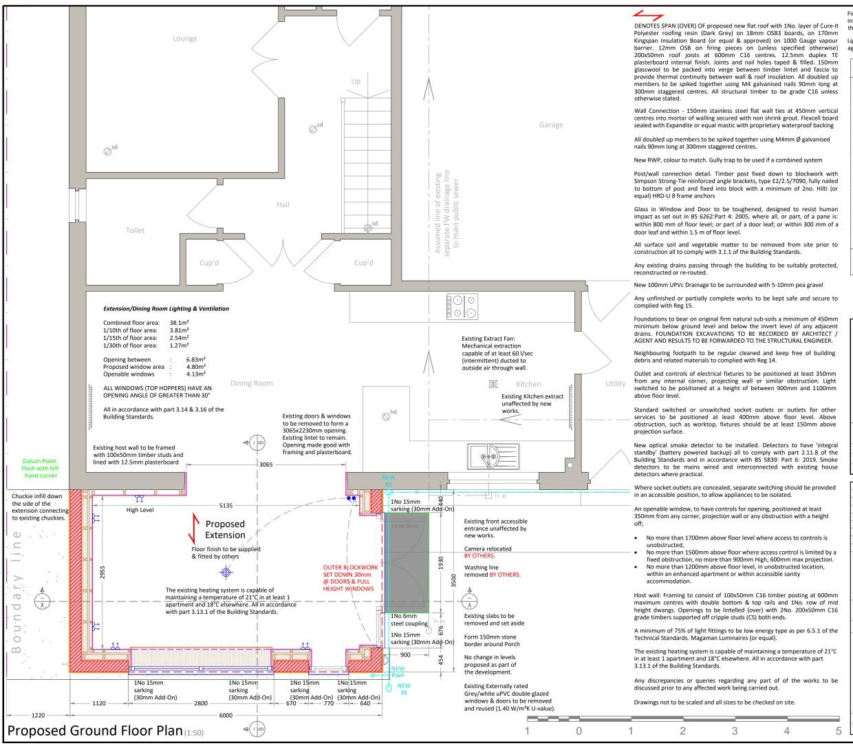
Final position of rad's to be agreed on site by customer. All new pipework insulated with foam pipe lagging to BS5422:2009. Rad fitted with thermostatic valve
