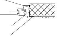
horizontal timber cladding support timber battens -
