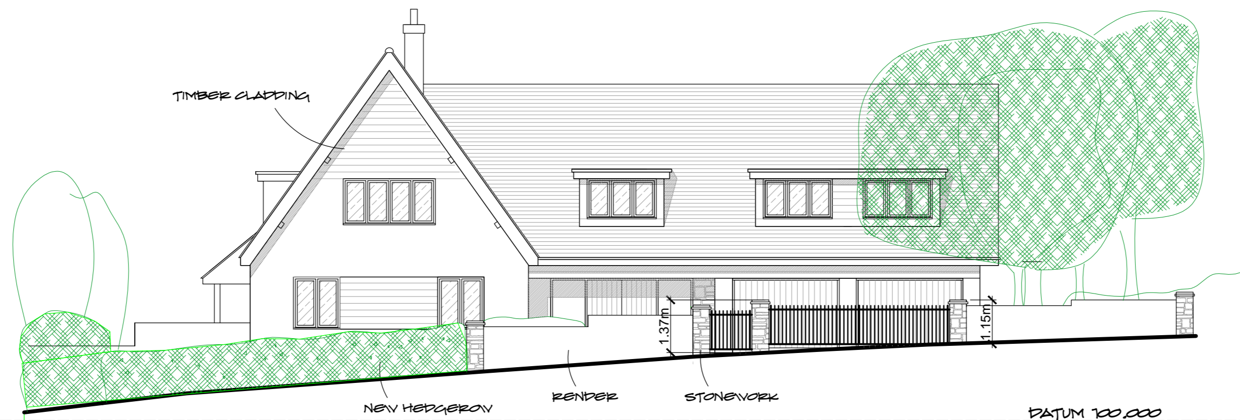
NORTH EAST ELEVATION OF PROPOSED BOUNDARY TREATMENT
