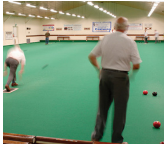
Example of high reflectance from ceiling and end walls as recommended by English Indoor Bowls Associations
