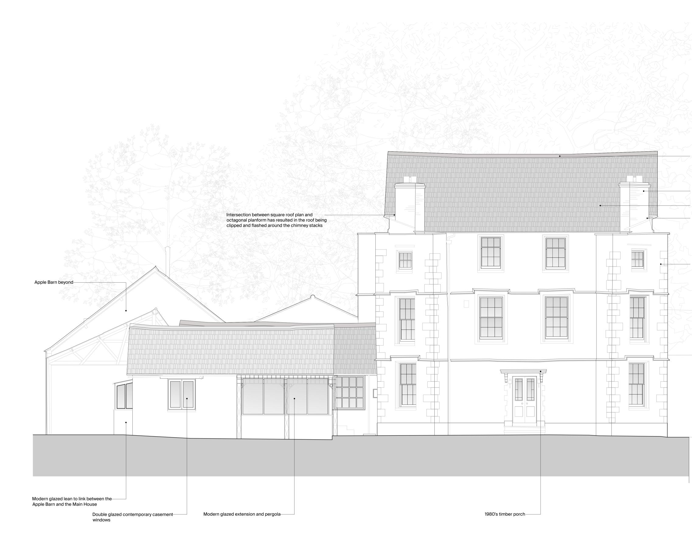
06 Existing West Elevation 1:50@A1, 1:100@A3
