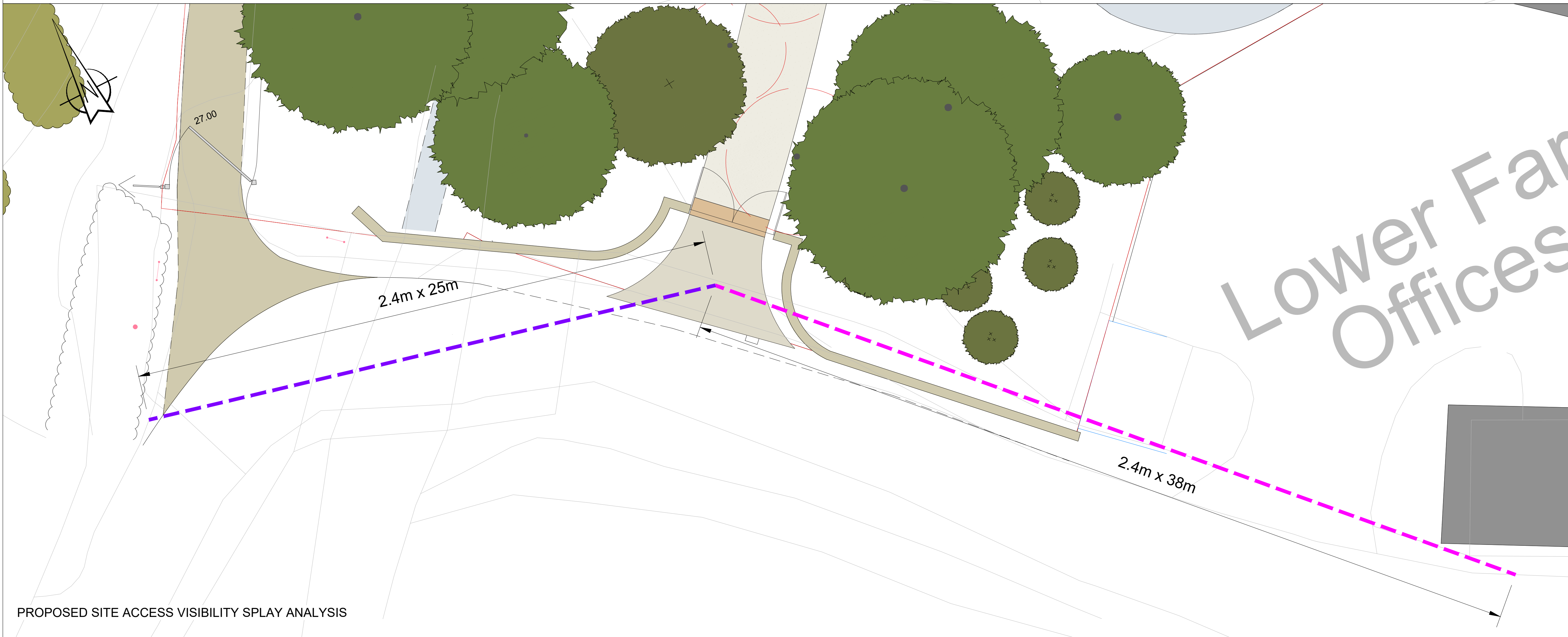
EXISTING SITE ACCESS VISIBILITY SPLAY ANALYSIS
