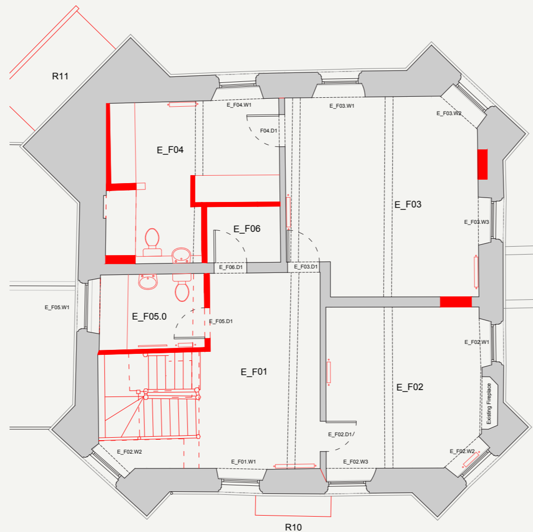
DEMOLITION FIRST FLOOR PLAN
