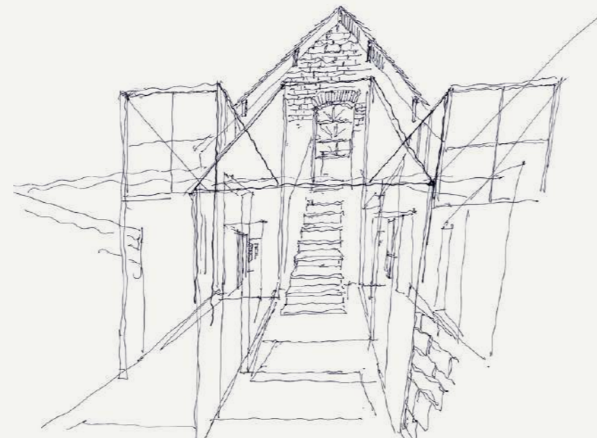
CONCEPT VIEW THE ROOF ANGLES OF THE PROPOSAL RESPOND TO THE THREE OPENINGS IN THE EAST FACADE
