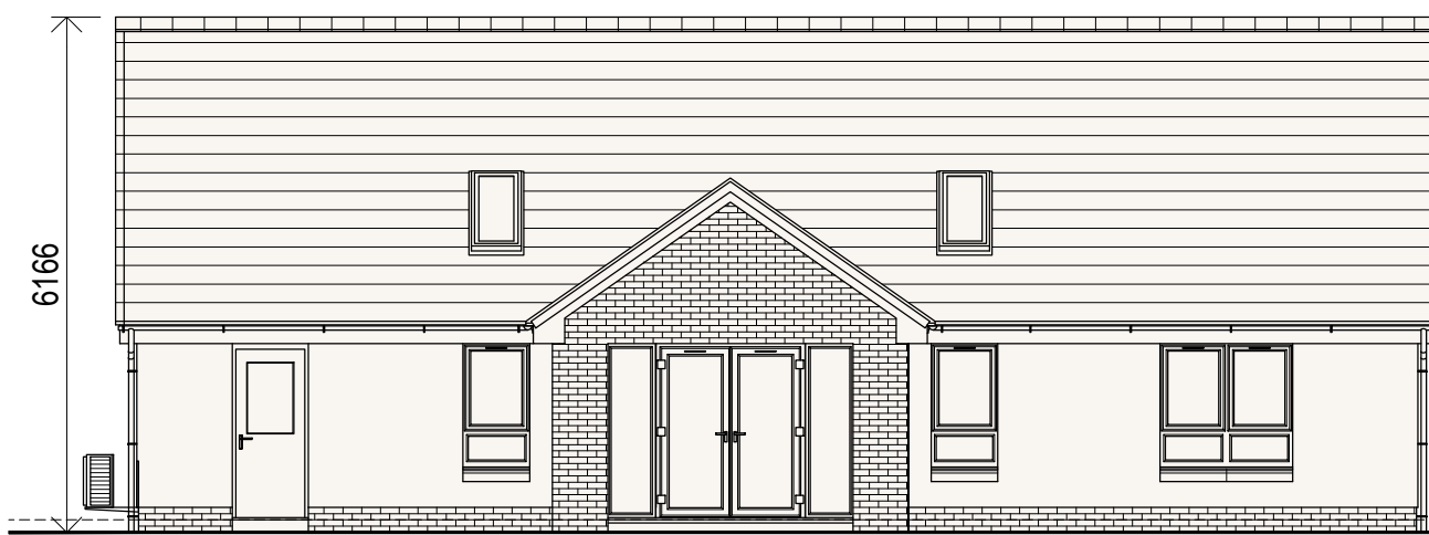
Rear Elevation 1:100 South Facing
