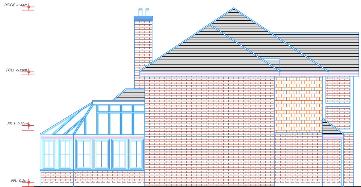
EXISTING SIDE ELEVATION A
