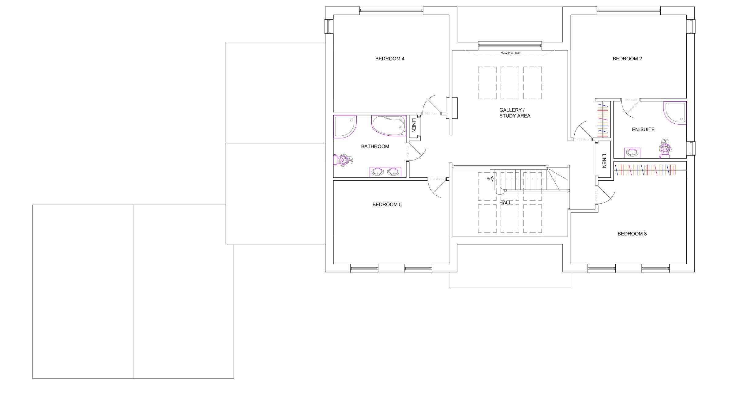
PROPOSED FIRST FLOOR PLAN SCALE 1:50 Do not scale for construction purposes.
