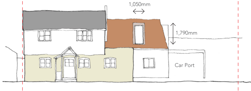
Street Elevations showing reduction in scale of dormer window from previous proposal (above) to current (below).
