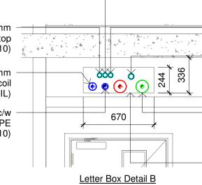
32Ø Conduit for TV 10mm QuelStop HPE Graphite Sealant (QHPE310) ■ 32Ø Conduit for Access Control 10mm QuelStop HPE Graphite Sealant (QHPE310)
