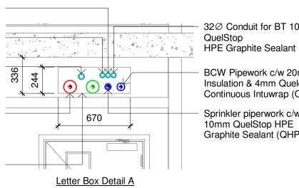
32Ø Conduit for TV 10mm QuelStop HPE Graphite Sealant (QHPE310) 32Ø Conduit for Access Control 10mm QuelStop HPE Graphite Sealant (QHPE310)
