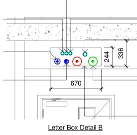
32Ø Conduit for TV 10mm QuelStop HPE Graphite Sealant (QHPE310) 32Ø Conduit for Access Control 10mm QuelStop HPE Graphite Sealant (QHPE310)  $40 \oslash$  Conduit for Submain 10mm QuelStop HPE Graphite Sealant (QHPE310)
