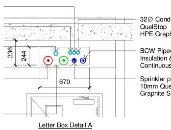
32Ø Conduit for TV 10mm QuelStop HPE Graphite Sealant (QHPE310) 32Ø Conduit for Access Control 10mm QuelStop HPE Graphite Sealant (QHPE310) 40Ø Conduit for Submain 10mm QuelStop HPE Graphite Sealant (QHPE310)
