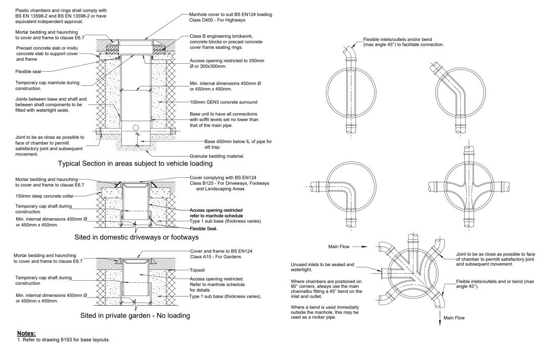
min. compressive strength 25 N/mm² (C25 concrete)
