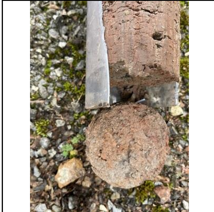
Photo OE/1702/1055/R2/P81 – Window Sample WS6 – Core at 3.0m bgl end.
