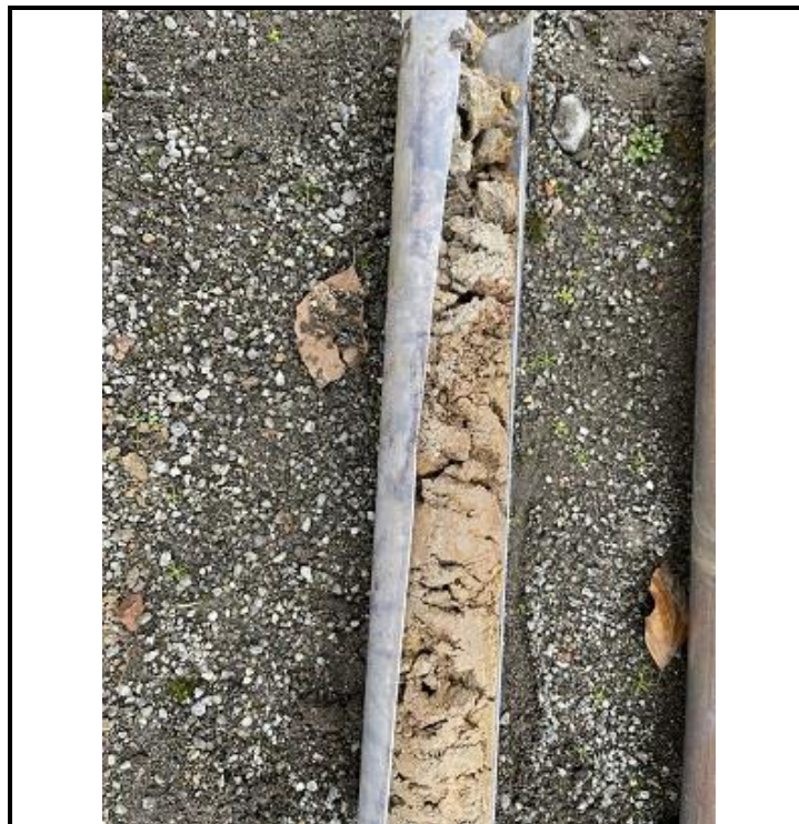
Photo OE/1702/1055/R2/P32 – Window Sample WS3 – Core 2.0 to 2.4m bgl
