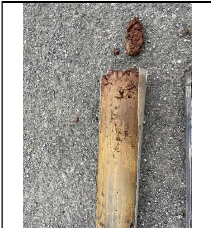
Photo OE/1702/1055/R2/P42 – Window Sample WS4 – Core 0.0 to 1.0m bgl
