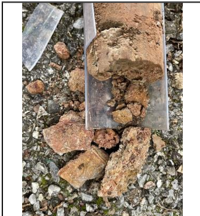
Photo OE/1702/1055/R2/P84 – Window Sample WS6 – Core at 3.8m bgl - end.
