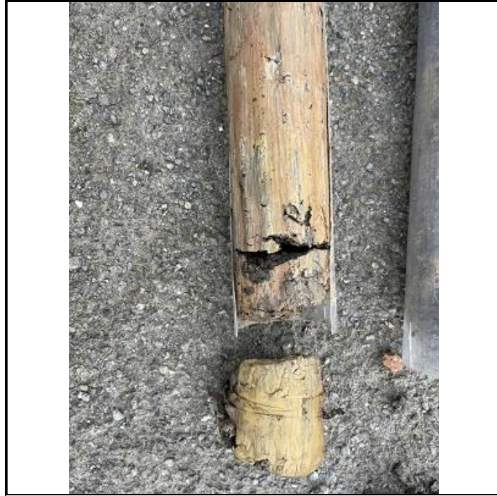
Photo OE/1702/1055/R2/P59 – Window Sample WS5 – Core 1.7 to 2.0m bgl.
