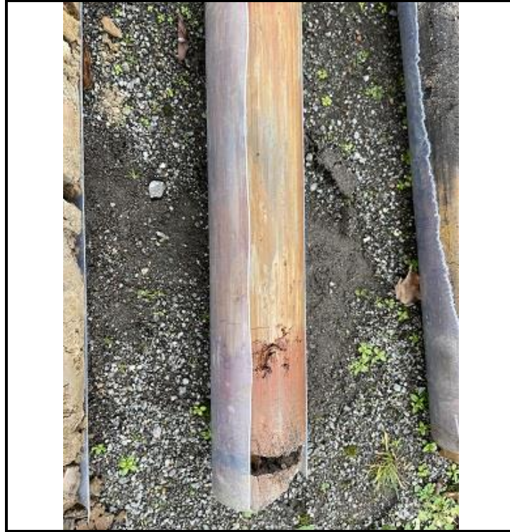
Photo OE/1702/1055/R2/P31 – Window Sample WS3 – Core 1.6 to 2.0m bgl
