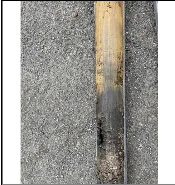
Photo OE/1702/1055/R2/P41 – Window Sample WS4 – Core 0.3 to 0.6m bgl
