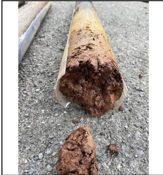
Photo OE/1702/1055/R2/P43 – Window Sample WS4 – Core 1.0m bgl – end.
