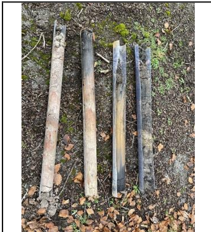
Photo OE/1702/1055/R2/P10 – Window Sample WS2 – Cores 0.0 to 4.0m bgl
