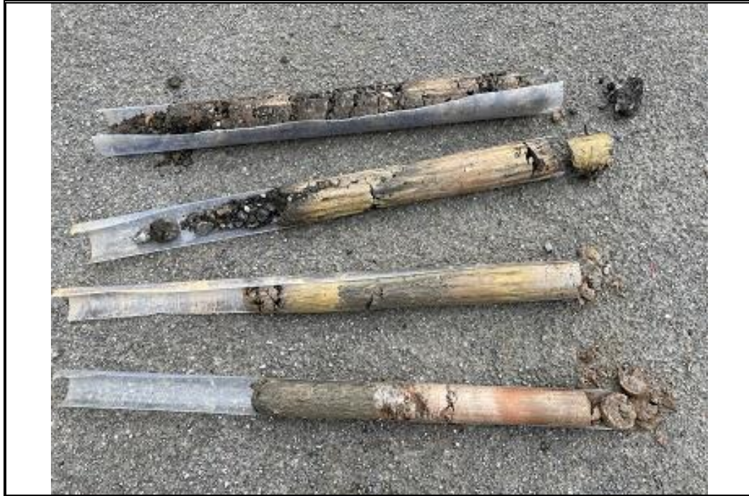
Photo OE/1702/1055/R2/P53 – Window Sample WS5 – Cores 0.0 to 3.5m bgl.
