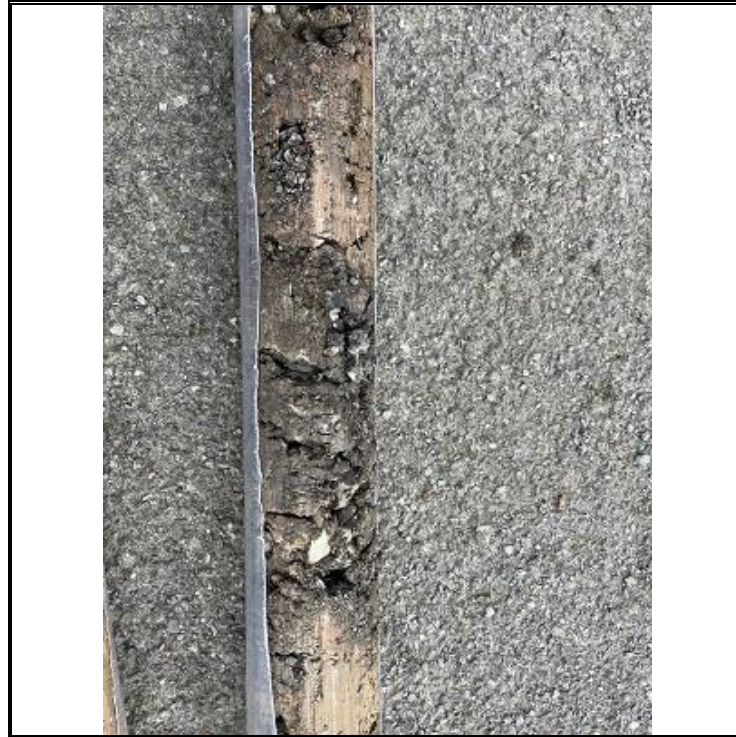
Photo OE/1702/1055/R2/P55 – Window Sample WS5 – Core 0.3 to 0.6m bgl.
