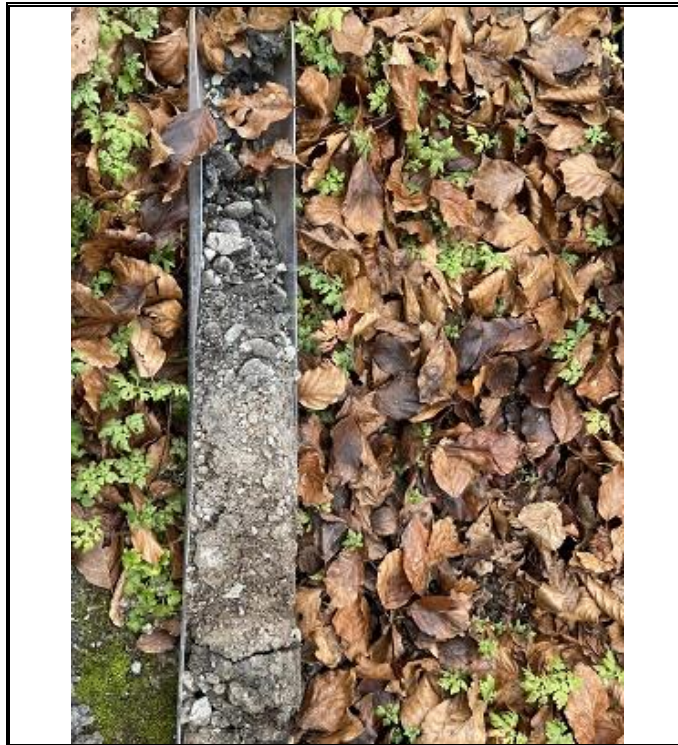
Photo OE/1702/1055/R2/P70 – Window Sample WS6 – Core 0.0 to 0.3m bgl.
