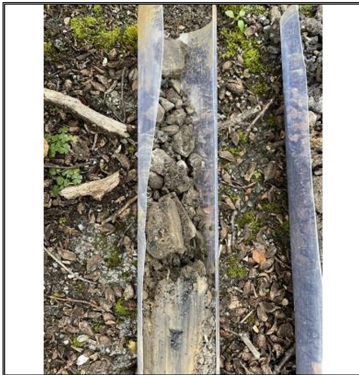
Photo OE/1702/1055/R2/P14 – Window Sample WS2 – Core 1.0 to 1.3m bgl
