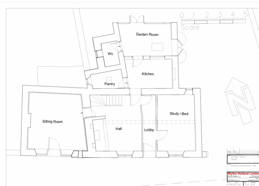
Figure 6. Existing ground-floor plan (Wythe Holland Ltd). The 'sitting room' was the Post Office. The kitchen and Post Office were among the additions of 1885 x 1899.
