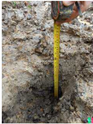
Plate 3 – Example of 350mm diggable soils in rear garden of Plot 174 with space for 150mm topsoil on top, taken 13/12/2023.
