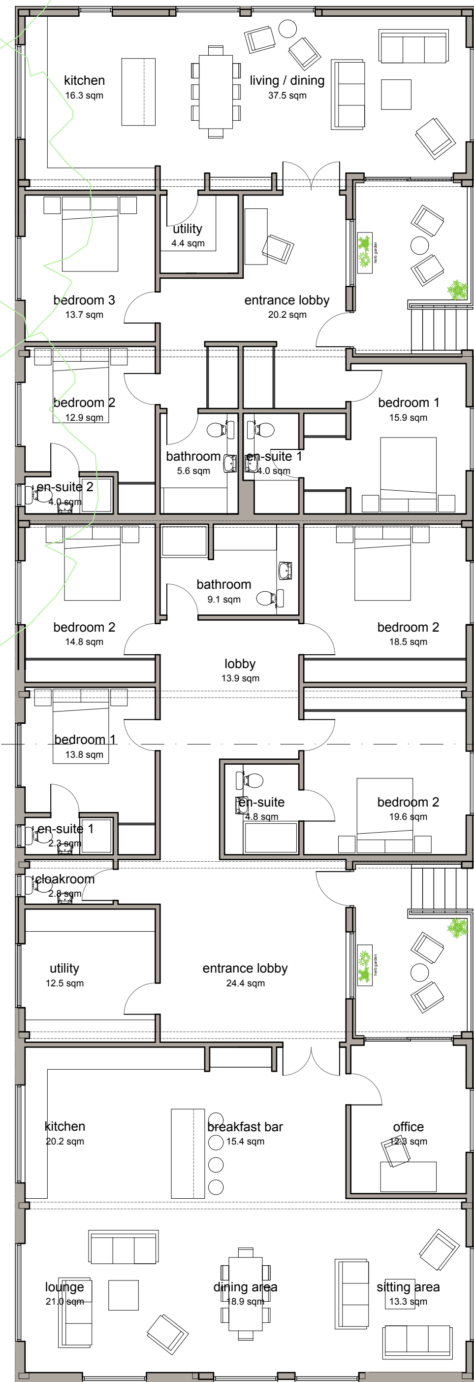
proposed ground floor plan plot 2, 1:100 Ground Floor Gross Internal Area = 141.9 sqm [1527 sqft]
