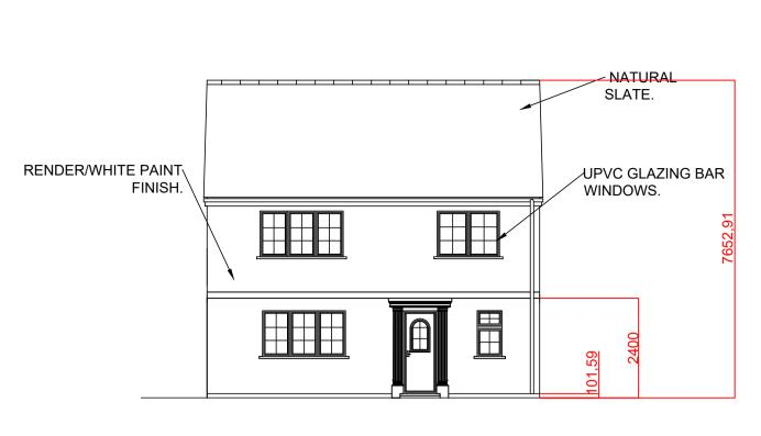
PROPOSED SOUTH/SW FACING ELEVATION SCALE @ 1:100.
