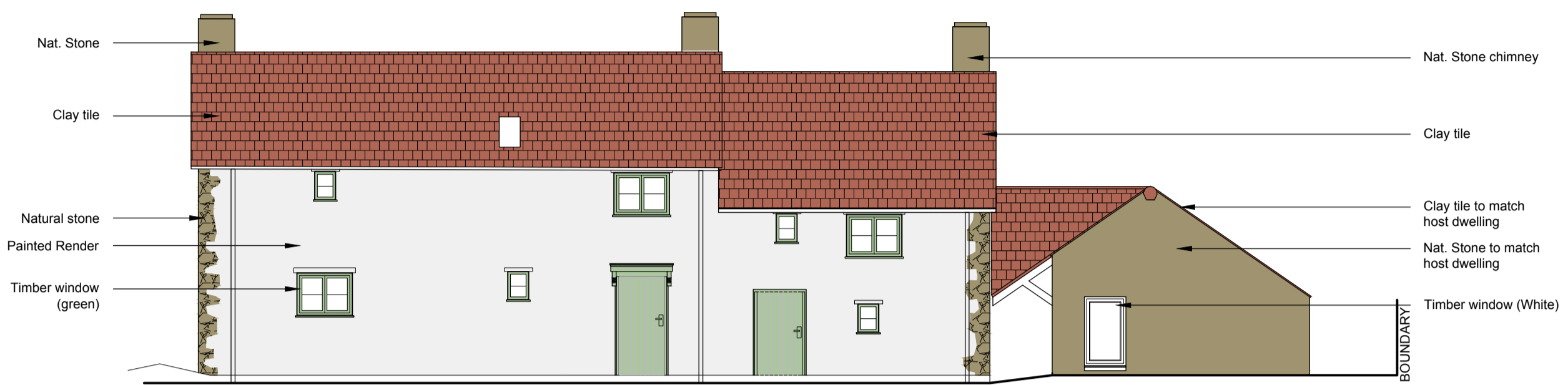
Northern Elevation (Street)
