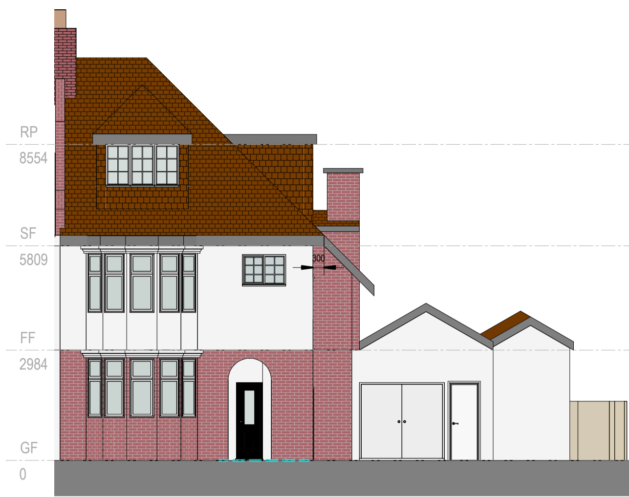
Front Elevation - Existing 1:100
