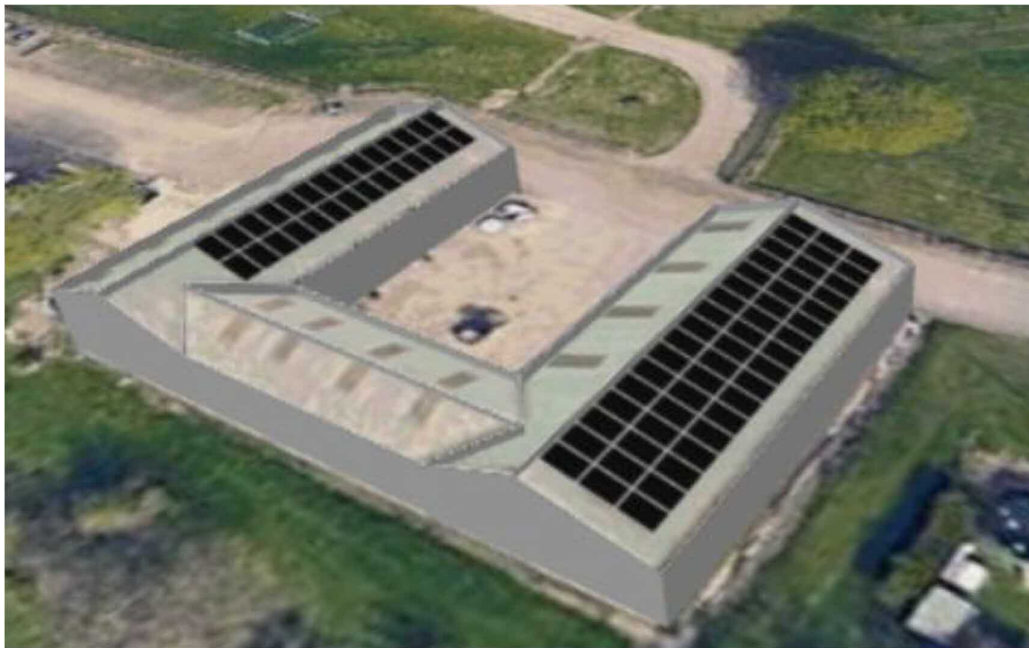
Figure 2 – 3D view of PV layout on MTS Grounds maintenance building's roof (courtesy of Powercor)
