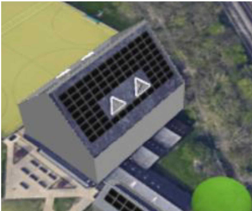
Figure 3 – 3D view of PV layout on MTPS Sports hall building's roof (courtesy of Powercor)
