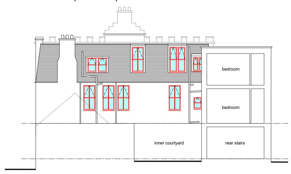
PROPOSED INTERNAL REAR (EAST) ELEVATION TO REAR BEDROOM BLOCK. 1:100.
