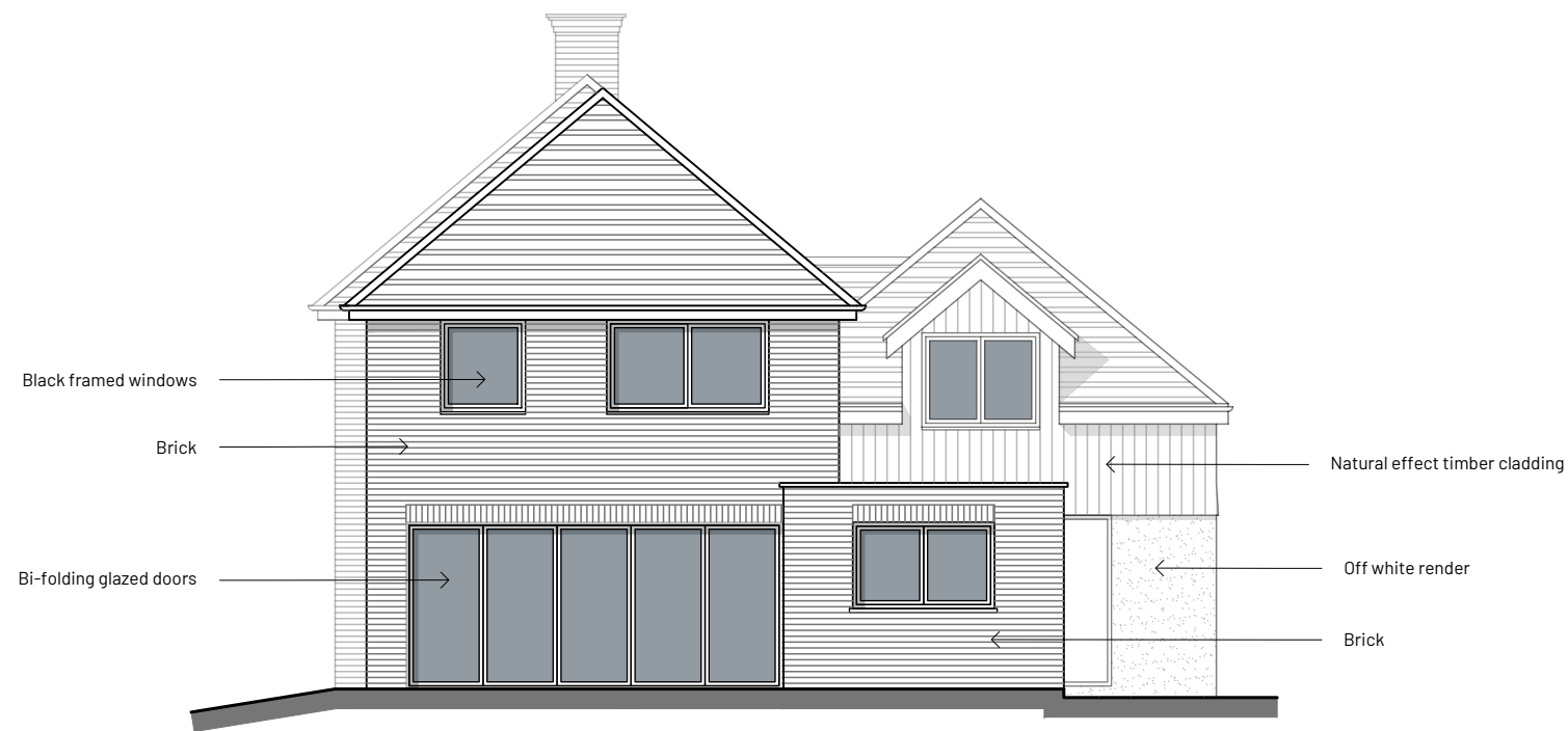
REAR ELEVATION (SOUTH FACING)
