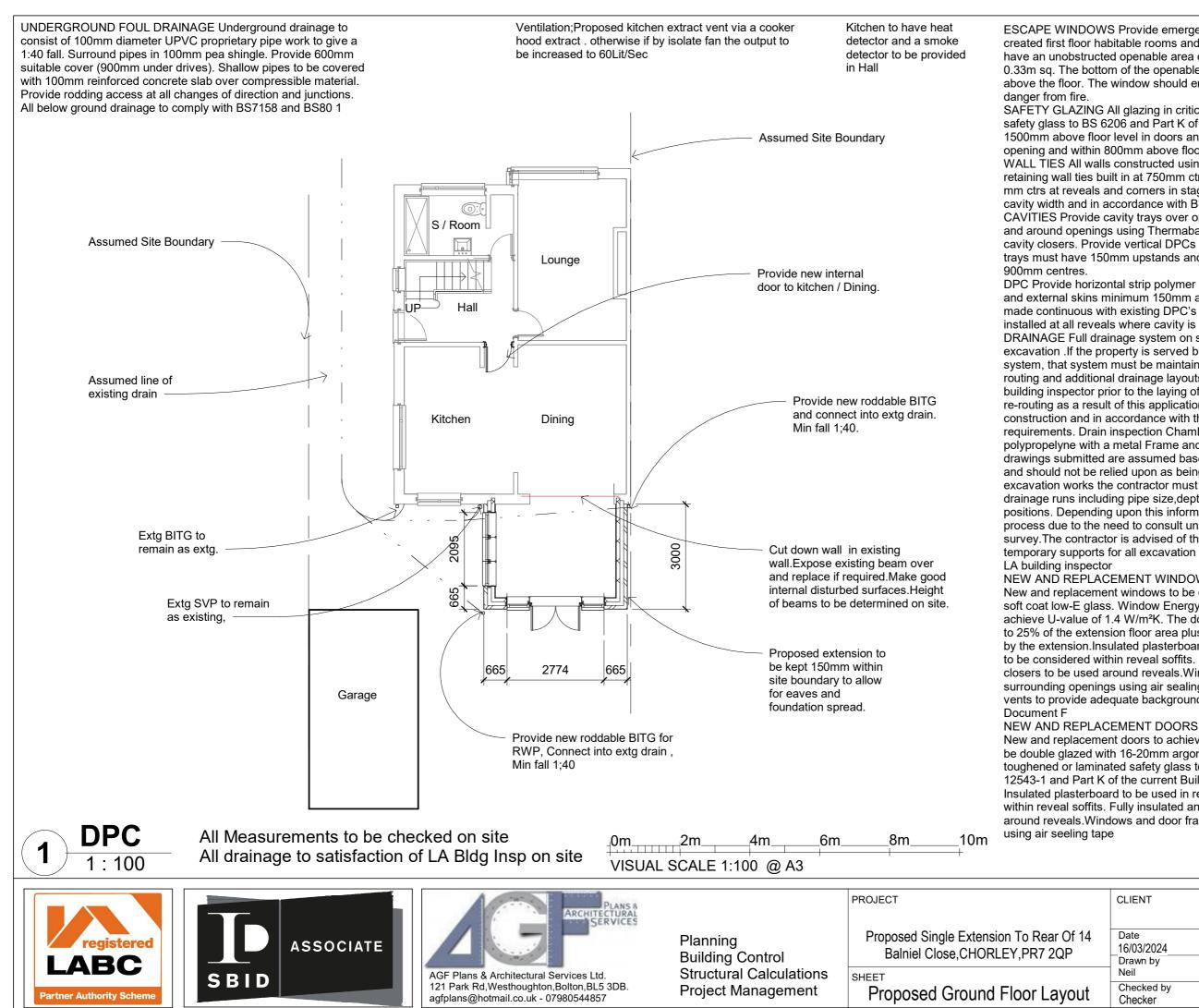
ESCAPE WINDOWS Provide emergency egress windows to any newly created first floor habitable rooms and ground floor inner rooms. Windows to have an unobstructed openable area of minimum 735x450mm, minimum 0.33m sq. The bottom of the openable area should be not more than 1100mm above the floor. The window should enable the person to reach a place free from
